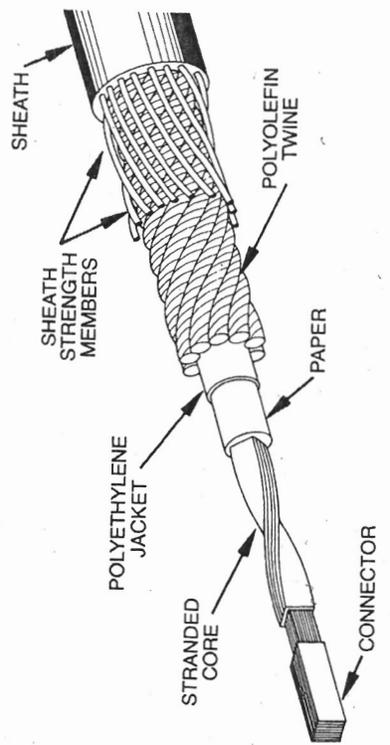
Fig. 20-46. The cable used in the Atlanta system contained 12 ribbons—each encapsulating 12 glass fibers.
