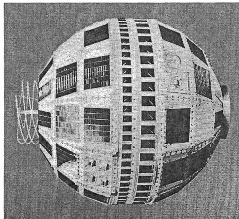
Fig. 13-5. The Bell System's experimental communications satellite, *Telesat I*, as it appeared before launch. Dark areas are solar cell arrays.
