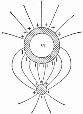
Showing induction and external field. Space S is completely shielded.
