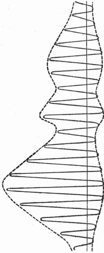
Single sideband, a modified form of amplitude modulation, takes up less band space than a regular AM signal. A sideband is eliminated—then replaced by the receiver (if it has a BFO/SSB control) when you tune it in. Single sideband is used extensively by utility stations, ham stations, some radio pirates, and a few international shortwave broadcast stations.
