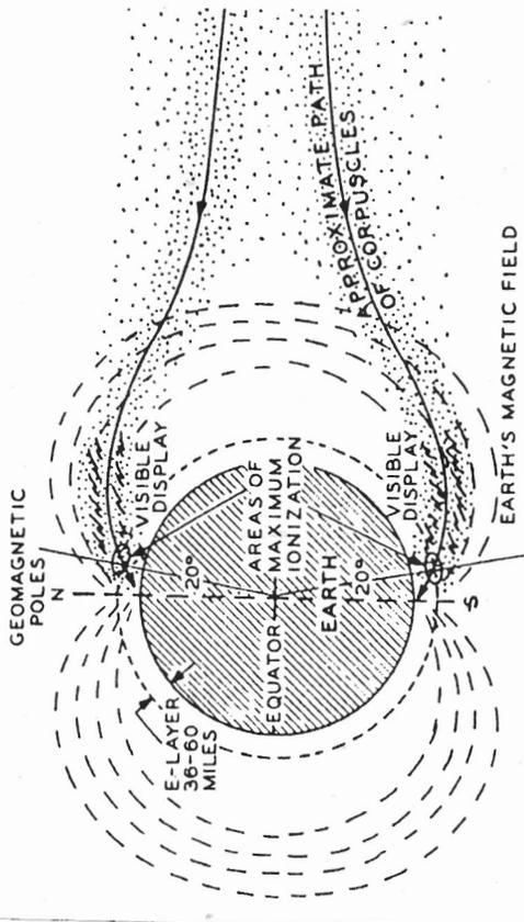
**Fig.18** Maximum aurora display is concentrated in a broad belt near 70 degrees latitude from each geomagnetic pole. The visible ionization occurs at a height of 60 to 70 miles in the E-layer of the ionosphere.
