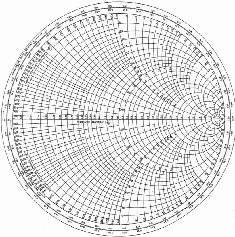
Fig. 3-12. The Smith chart transmission-line calculator. By means of the chart, the input impedance and standing-wave ratio may be determined for a transmission line of any length terminated in any impedance. [Smith, *Electronics* 12 (1939): 31.]
