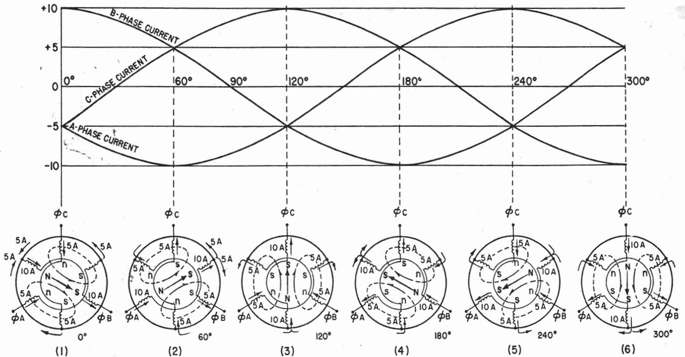
Figure 17-1.—Development of a rotating field.
